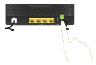
4 The (1) LED turns on. Wait at least two minutes to allow your TG588v v2 to complete the startup phase.
