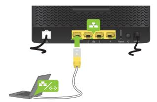
2 Connect the other end of the Ethernet cable to your network device.
